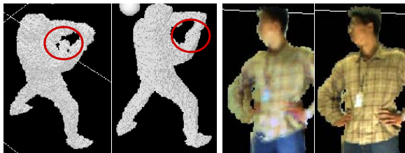
(a) Reconstructed 3D model (b) Texture mapping Fig. 1. Final results (without / with inner cameras)
